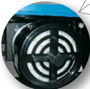
Positive displacement, motor-driven gear pump offers a continuous pulse free output.
