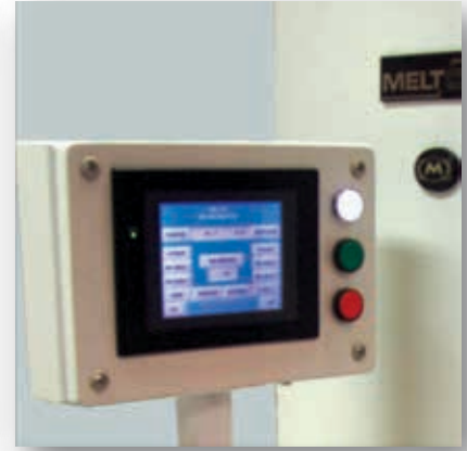
Touch-screen panel for operation
