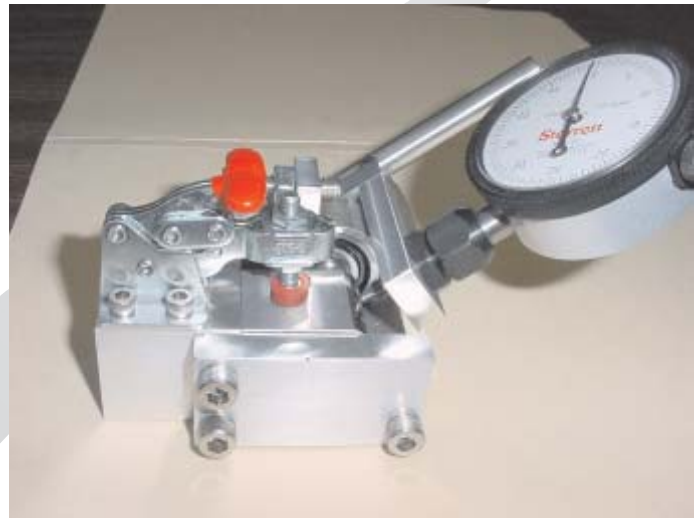
Fig. 2 – Measuring fixture for establishing the degree of wear on each applicator head
