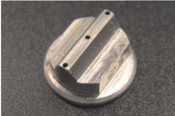
Typical non-contact adhesive nozzle
