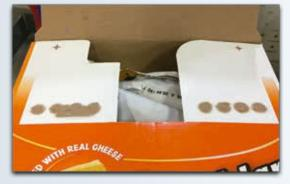
EcoStitch applies precision dots of adhesive in place of traditional lines or short line stitch. The EcoStitch system doesn't produce "angel hair" and has zero dynamic seals in the applicators therefor eliminating parts changes and usage of items such as nozzles, air solenoids and glue modules.
