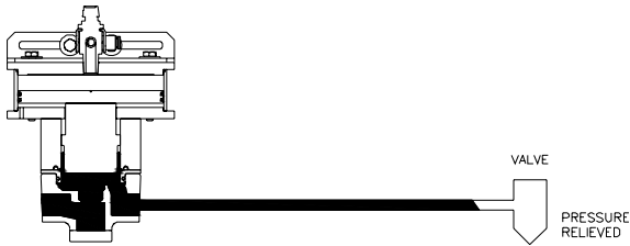
No Pressure (Machine Stopped)
