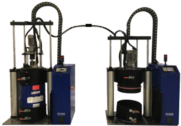
Two units can work in tandem; when the first unit is empty, it automatically switches to the second unit.
