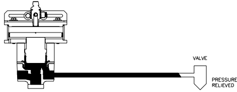
No Pressure (Machine Stopped)
