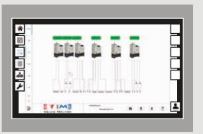
Smart Control allows the operator to visualize and manage the complete hot melt dispensing system (drum unloaders, melters, applicators, and accessories). Easily control your working process, create recipes, modify parameters, and program alarms. The system also generates and displays adhesive usage reports and simplifies maintenance monitoring with scheduled notifications when maintenance or replacements are required (resistors, modules, pumps, filters...).
