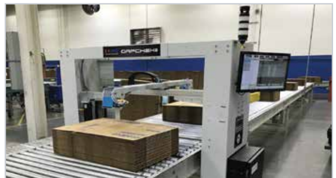
Inspects every finished manufacturer's gap
