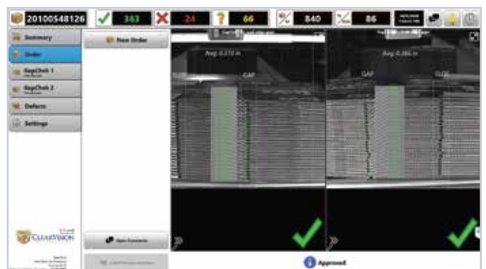
Illustrates each individual gap measurements through familiar ClearVision user interface
