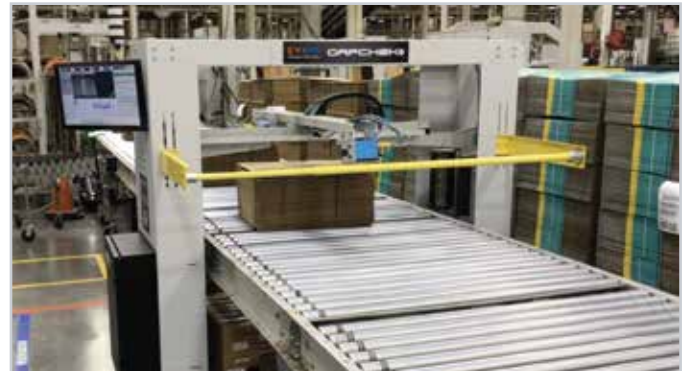
Mounts over existing flat top or roller style conveyor
