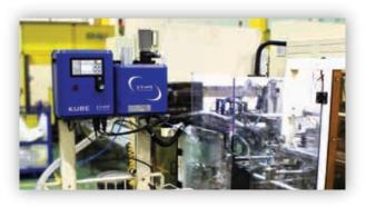
Engineered to operate with three different mount configurations, Kube Zero is suitable for both new machine installations, as well as system upgrades/replacements.
