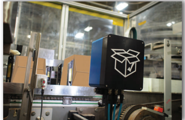
PackChek™ installed on a cartoning machine with a hot melt gluing system
