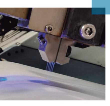
Valco Melton's Alpha Spray Nozzle guarantees a cleaner spray pattern with an excellent edge control, ideal for continuous laminating applications. It helps to drastically reduce adhesive contamination around the application
