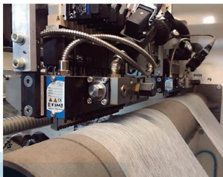
The main advantage that we provide is that we have inserts with 6 air orifices per adhesive stream for a higher frequency on the swirl, which allows customers benefit from a higher bonding as the number of crossing points of the swirl pattern increases. This feature also allows the end users to run the machine at
