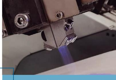
Valco Melton's Sigma Nozzles have been specially designed for high-speed intermittent applications, to prevent adhesive bleed-throughs and thermal distortion during intermittent adhesive applications, especially when used to bond thin materials, reducing associated machine downtime and helping to improve product quality.
