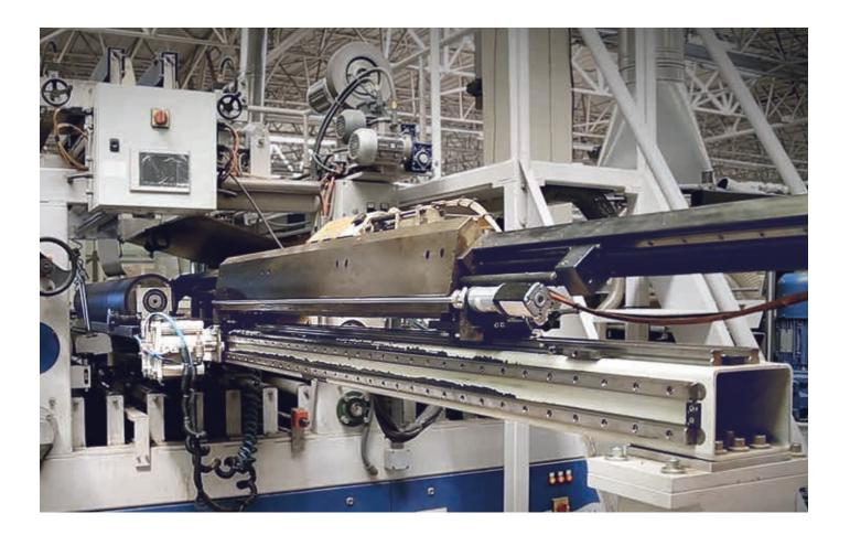
No scratches. Rotating bar eliminates contaminants trapped between applicator and substrate
