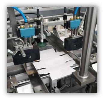
The MK-F Gun Series offers two module options: *bead* or *zero cavity*. *Bead* mini modules work with standard straight, 90° and spherical nozzles. *Zero cavity* mini modules provide extremely fast and accurate pattern placement with any adhesive type.
